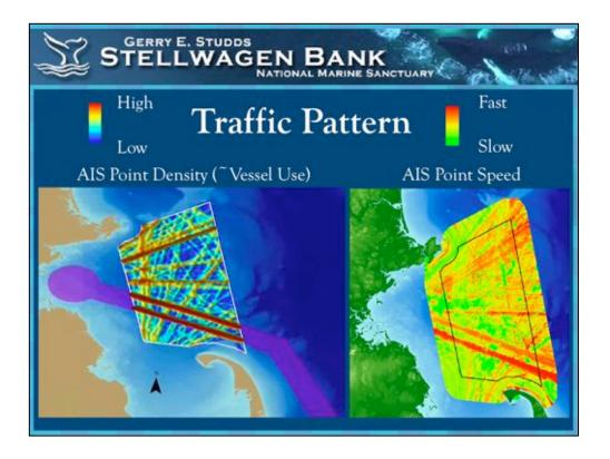
AIS can give a clear picture of traffic patterns. The density of vessel use is shown on the left and speed of vessels is shown on the right. One can clearly see the high use through the shipping lances.
