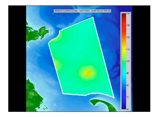
This slide shows intensity of vessel traffic, recorded from on unit in the sanctuary, over a 24 hour period.
