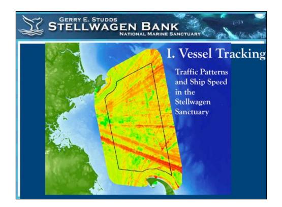
Beginning with information that we can gain from vessel tracking: the use of AIS (automatic identification system) data allows us to look at traffic patterns for all large commercial vessels over **300 gross tons or carrying more than 165 passengers**.
