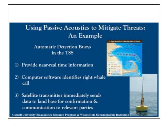
Real-time acoustic detections in the Boston area utilize surface buoys called automatic detection buoys, developed by Cornell University's Bioacoustics Research Program and moorings developed by Woods Hole Oceanographic Institution....
